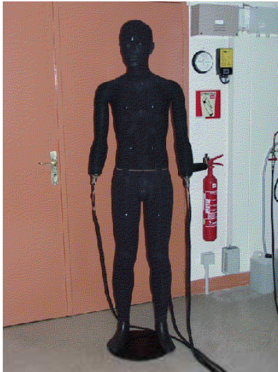
Figure 1: The instrumented thermal and sweating manikin.
