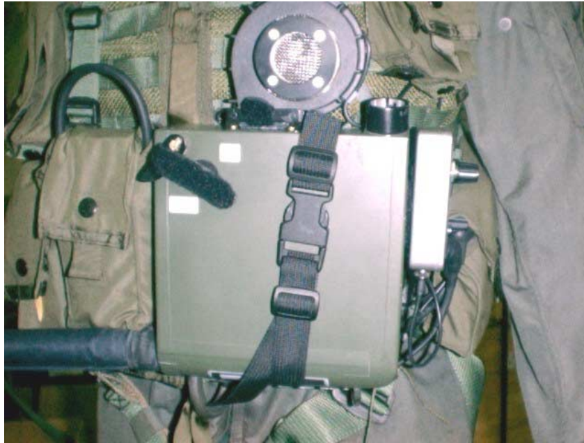
Figure 8: APACS FM Arrangement on AIRSAVE Vest
